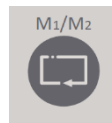
Figure 48. The left push-button shifts between readings/counts of the two flow sensor inputs. In the display, M1 and M2 respectively indicate the currently displayed flow sensor inputs/counters.
