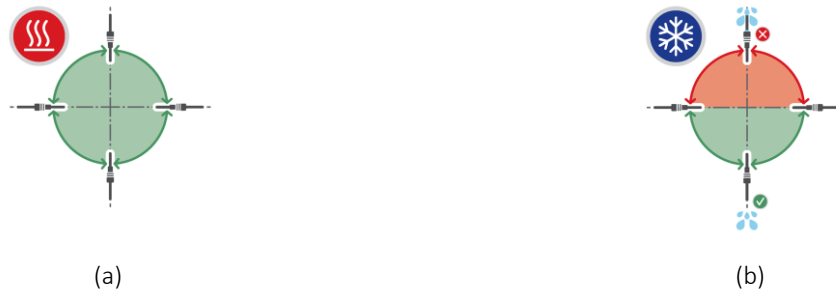
Figure 19. Acceptable orientation of a temperature sensor in (a) a heating and (b) a cooling installation.
