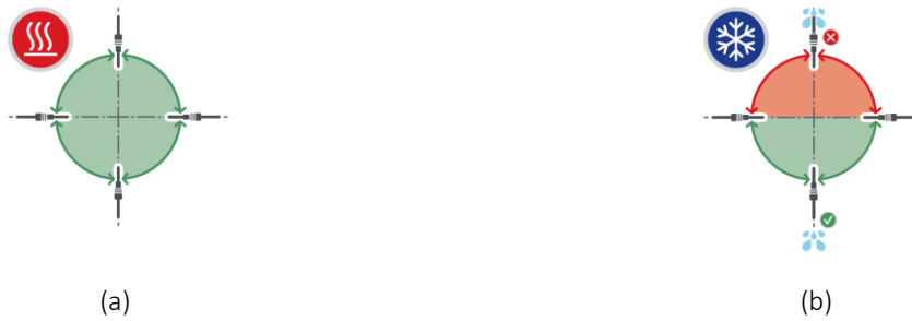
Figure 19. Acceptable orientation of a temperature sensor in (a) a heat and (b) a cooling installation.
