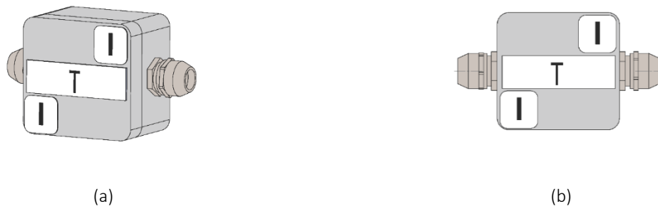
Figure 70. Sealing of Cable Extender Box seen from the side (a) and from the front (b).
